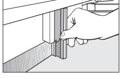
■ Wedge the air separator at the bottom of the freezer door, so it connects in place.
